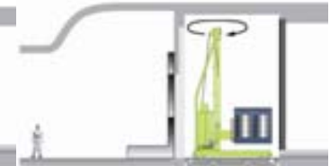
Rotating the lifting machine on the moveable floor with turntable
