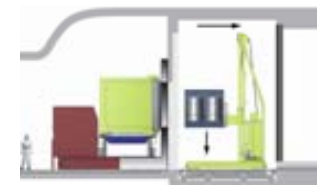
Moving the lifting machine to the moveable floor and lowering the package
