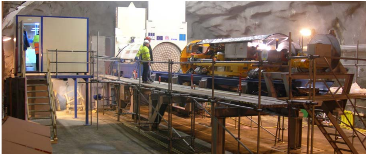
Figure 2. Set-up of equipment at the test site at Äspö HRL, level -220m. The Super Container is inside the transport tube with the radiation shielding gates open. The control room is on the left side on this photo.
