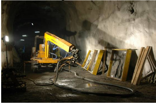
Fig. 2: Spraying tests on Opalinus Clay panels.
