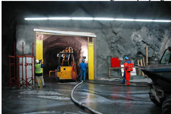
Fig. 3: Horseshoe tunnel profile for the large-scale field test.
