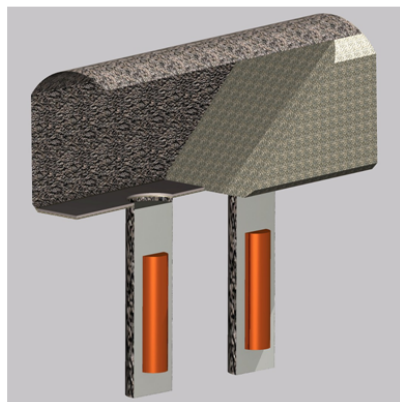
Figure 1. Schematic picture of the engineered barrier system of the KRS.
