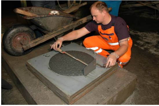
Fig. 1: Fresh concrete test (flow table test) of LPH shotcrete (wet mix).
