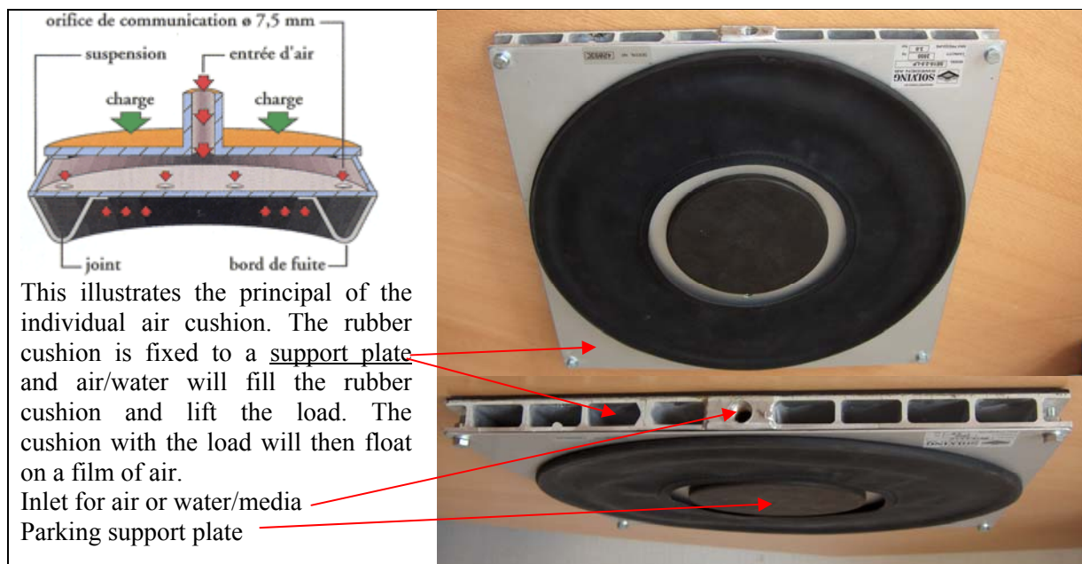
Figure 1. Illustration of the design of an air cushion.
