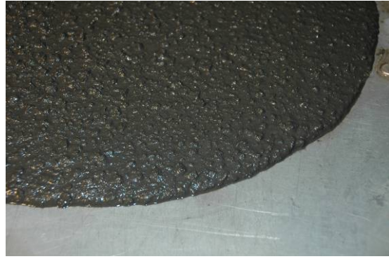
Fig. 1: Fresh concrete test (flow table test) of LPH shotcrete (wet mix).
