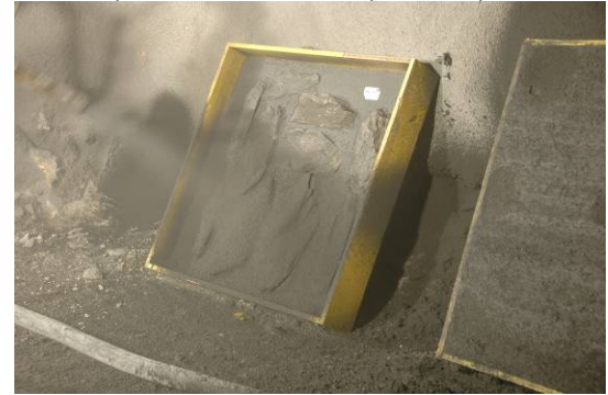
Fig. 2: Spraying tests on Opalinus Clay panels.
