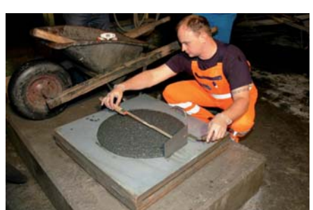
Low pH shotcrete applied on test panels of Opalinus Clay
