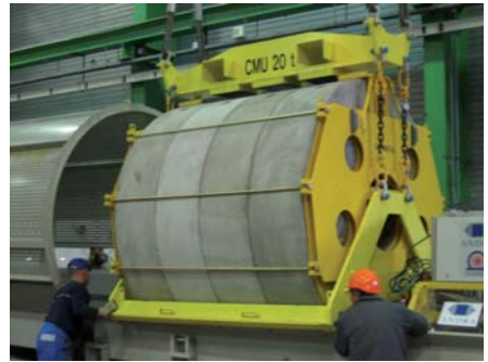
View of set of 4 rings loaded onto air cushion test bench launch table (fabricated as part of Module 3)
