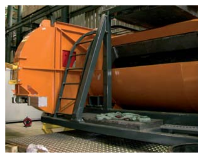
Shielding cask door frame and viewing window
