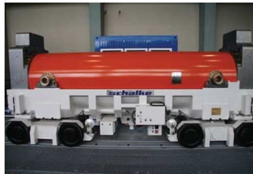
Newly fabricated transport cart and transfer cask
