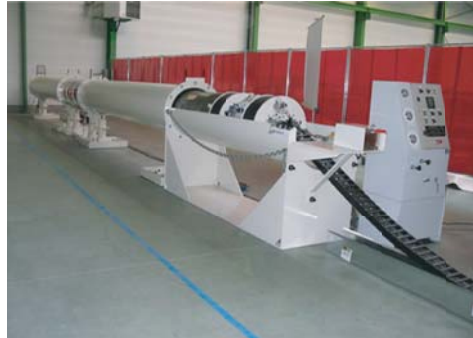
Andra's prototype pushing robot test bench set up at Musthane Lille / France October 2005
