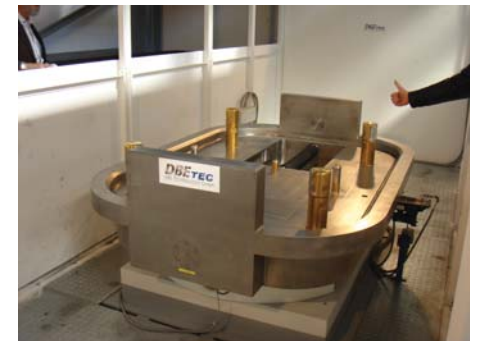
Newly fabricated borehole lock installed in borehole cellar
