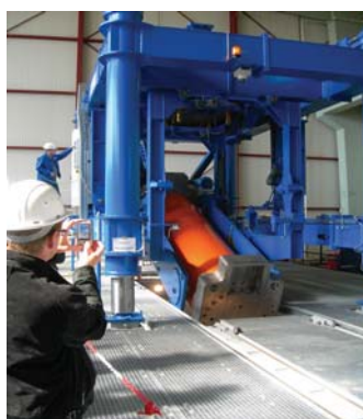
Emplacement device swivelling the transfer cask into an upright position
