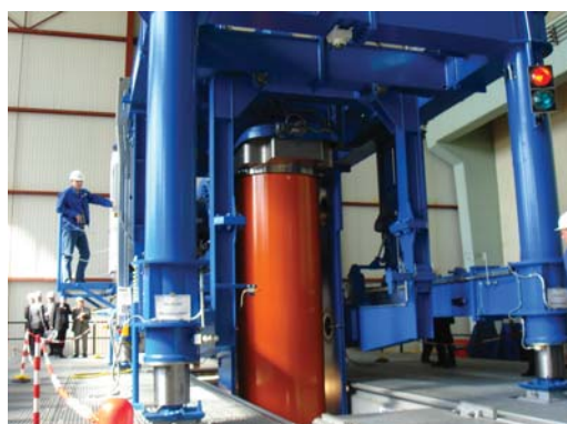
Emplacement device lowering down the transfer cask
