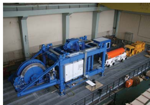
Vertical emplacement device set up in demonstration facility at Landesbergen
