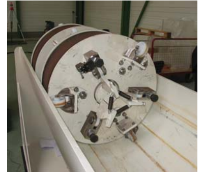
Front view of first pushing robot showing 3 fingers for gripping canister and 2 inflatable toric jacks
