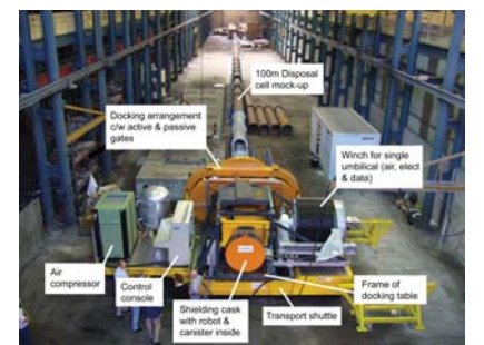
Test bench set up at Saint-Chamond
