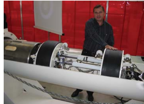
First full scale prototype pushing robot in extended position showing also canister and ceramic sliding runner
