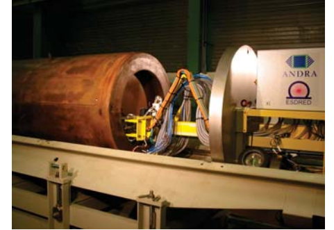
View showing emplacement cart, radiation shield, pushing jack, canister and gripping mechanism
