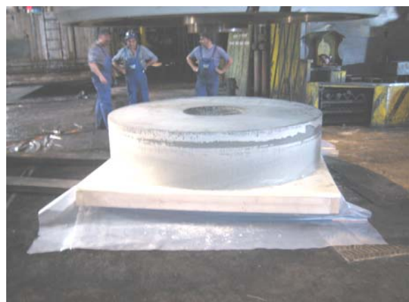
Figure 2: 4 Ton, 2.25m diameter bentonite/sand ring after 45 000 tons of pressure & stripping from mould (Andra)
