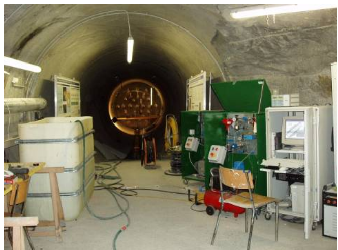
Figure 11: Long Plug in Background with Monitoring Equipment at Grimsel (Enresa / Aitemin / CSIC)
