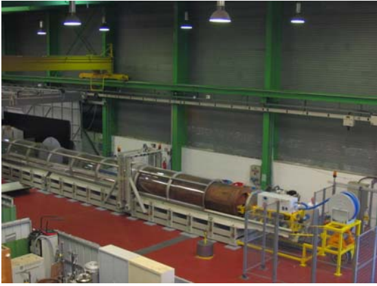
Figure 8: Demonstration of emplacement of 43 ton Spent Fuel canister using Air Cushion Emplacement Equipment (Andra)
