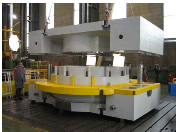
Figure 1: 100 Ton Mould for Pressing Sand/bentonite Rings (Andra)
