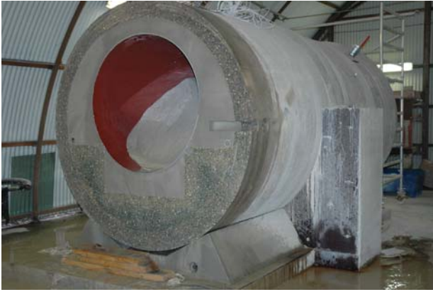
Figure 3: Reduced scale mock-up after backfill testing (Ondraf/Niras & Euridice)
