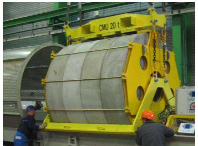
Figure 3: Andra - View of Dummy concrete rings loaded on air cushion test bench launch table
