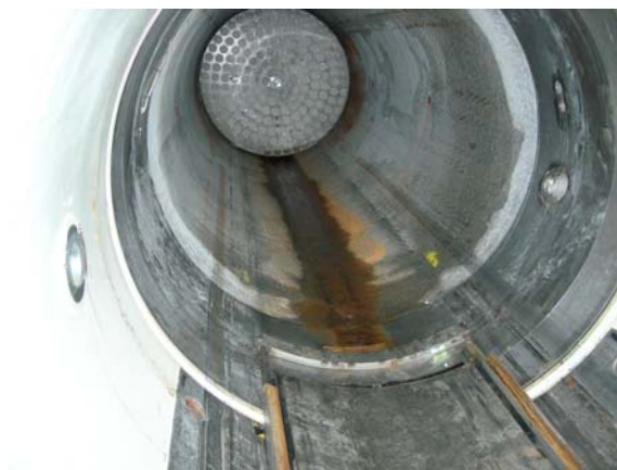
Figure 7: SKB - View of KBS-3H emplaced in the Äspö test drift during the SAT in Feb. 2007
