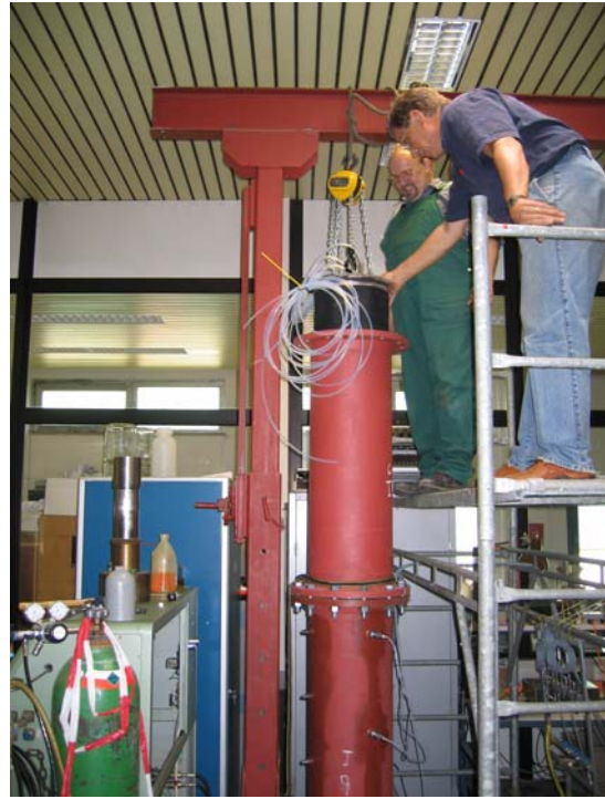
Figure 3 Mock-up test in GRS's geotechnical laboratory (left: test set-up, right: packer installation)
