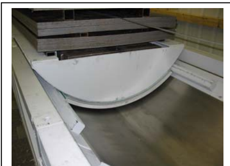
Figure 5 : Prototype test of the air cushion principle applied to a small diameter canister
