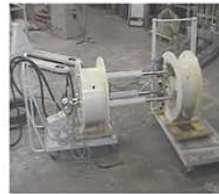
Frame of Andra's prototype pushing robot in extended position (length : 1m)
