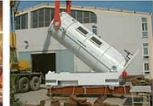
SKB's transport tube for super-container KBS-3H (45 ton)
